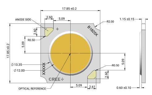
Tc measurement point: either the anode or cathode solder pad
