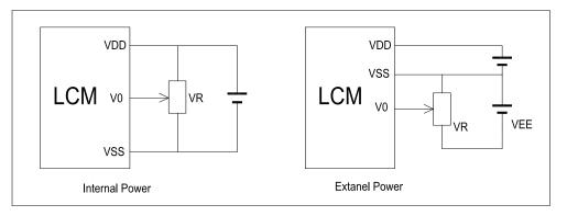
$V_{DD-V_0}$ : LCD Driving voltage VR: 10k~20k
