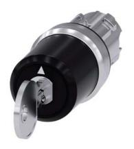
key-operated switch Siemens, 22 mm, round, metal, shiny, lock number SSG10, with 2 keys, 3 switch positions I-O<II, left latching, momentary contact type on the right, actuating angle  $2x45^\circ$ , 10:30h/12h/13:30h, key removal I, with laser labeling, inscription or symbol customer-specific selection with SIRIUS ACT configurator (CIN)
