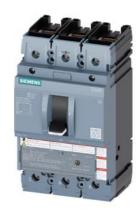
circuit breaker 3VA5 UL frame 250 breaking capacity class H 65kA @ 480 V 3-pole, line protection TM230, FTAM, In=80A overload protection Ir=80A fixed short-circuit protection Ii=5...10 x In UL489 SB (naval), 50 deg. cel. cable connection on both sides
