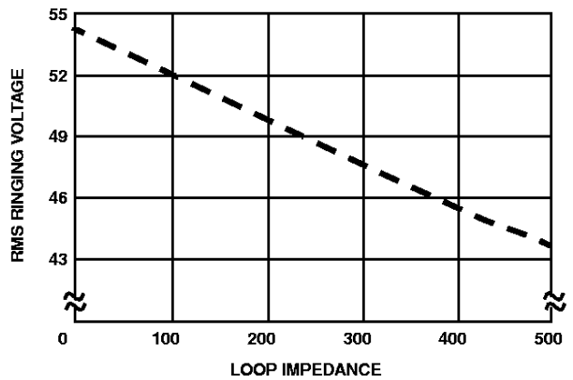
FIGURE 14. RMS RINGING VOLTAGE vs LOOP LENGTH REN = 4
