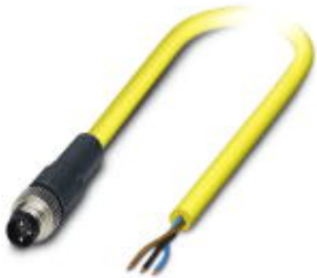
Sensor/Actuator cable, 3-position, PVC, Yellow RAL 1021, Plug straight M8, on Free cable end, Cable length: 2 m
