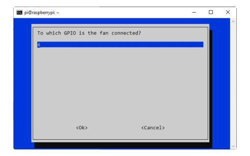
The default GPIO pin is 14, but the BrainCraft Hat has the fan connected to pin 4.
