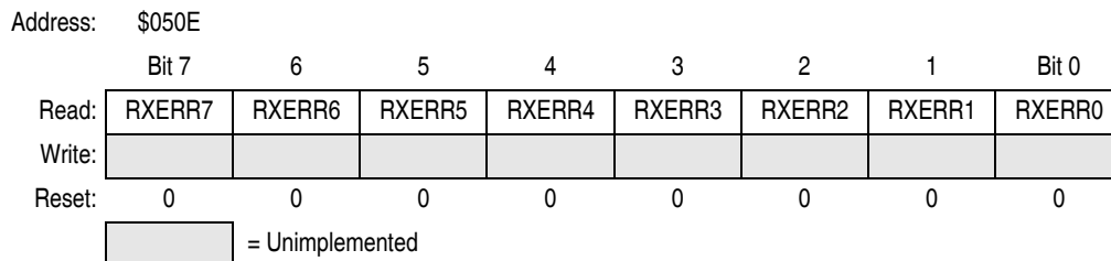
Figure 12-25. Receiver Error Counter (CRXERR)
