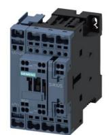
Contactor, AC-1, 35 A/400 V/40  $^\circ\text{C},$  S0, 4-pole, 24 V DC, 1 NO+1 NC, Spring-type terminal
