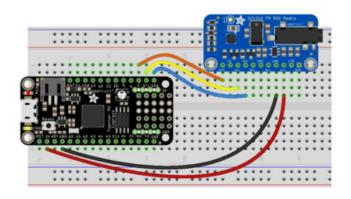
Board 3V to sensor VIN Board GND to sensor GND Board SCL to sensor SCL Board SDA to sensor SDA Board D5 to sensor RST
