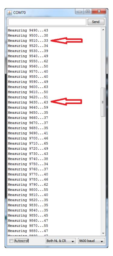
The larger the number the higher the transmission power. For example, 96.3MHz is a higher number than the others (FYI, its Univision 96.3 FM ()!) whereas 95.1 MHz is nice as low, that's not used for any transmission. Try to find a number that's also not surrounded by high numbers, since it can get 'drowned out' by the nearby frequencies.
