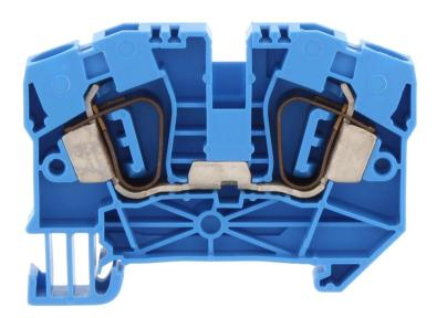
Ex feed-through terminal ATEX-certified, Tension-spring connection, Mounting type: Mounting rail TS 35/7.5, Rated cross-section: 6 mm², Width: 8.1 mm, Colour: Blue
