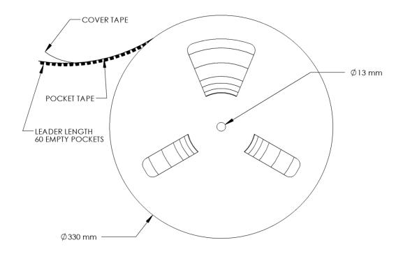
Figure 12: Emitter Reel specifications (mm).
