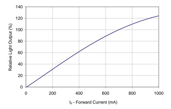
Figure 7: Typical relative light output vs. forward current @  $T_c = 25^{\circ}C$ .
