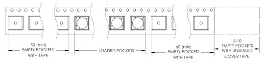
Figure 11: Emitter carrier tape specifications (mm).
