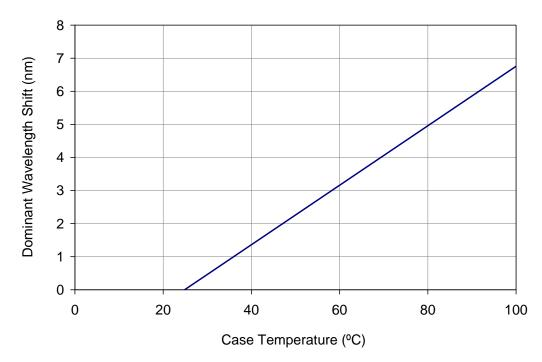
Figure 6: Typical dominant wavelength shift vs. case temperature.
