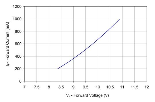
Figure 9: Typical forward current vs. forward voltage @  $T_c = 25^{\circ}C$ .
