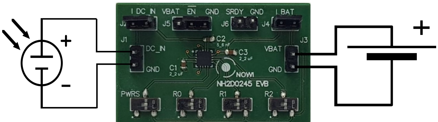
Figure 3: Connecting a harvester and battery
