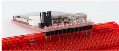
Pins soldered onto the imp Breakout Board
