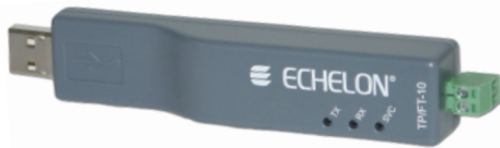
U10 USB Network Interface – TP/FT-10 Channel
