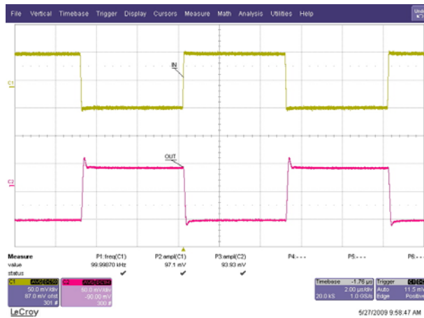
Figure 13. Inverting Small Signal Step Response
