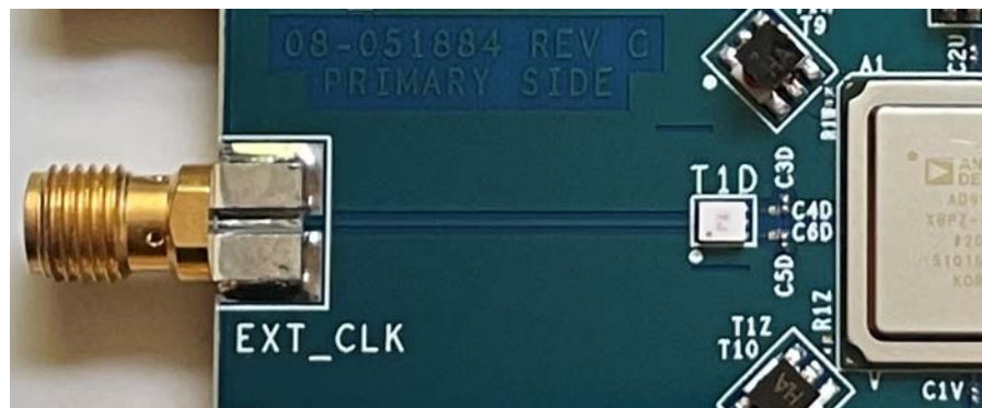
Figure 19. Capacitor Position for Direct External vs. On-Board HMC7044 Clocking (Showing the AD998x-FMCA-EBZ Evaluation Board)
