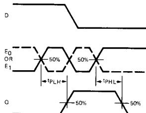
PROPAGATION DELAY ENABLE TO OUTPUT
