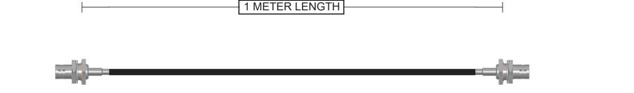
Connector A 112234 BNC Jack Straight Bulkhead - Rear Mount Brass Nickel 50 Ohm RG-174 Continuity/Hi-Pot Connector B 112234 BNC Jack Straight Bulkhead - Rear Mount Brass Nickel
