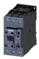
Contactor, AC-3, 37 kW / 400 V, 1 NO + 1 NC, 110 V AC, 50 Hz / 120 V, 60 Hz, 3-pole, Size S2, screw terminal
