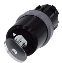
key-operated switch Siemens, 22 mm, round, plastic with metal front ring, lock no. LSG1, with 2 keys, 2 switch positions O-I, latching, actuating angle 90°, 10:30h/13:30h, key removal O, with laser labeling, lower case
