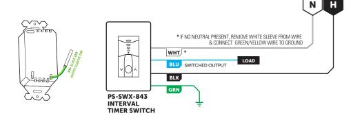
NOTE: This product is UL listed and meets NEC 404.2(c) & 404.22 guidelines regarding powering over ground & current leakage. Powering over ground is permitted for replacement / retrofit only.
