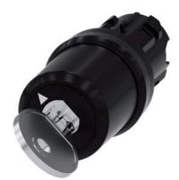
Key-operated switch BKS, 22 mm, round, plastic, lock No. E9 (VW), without key, 2 switch positions O-I, latching, actuating angle 90°, 10:30h/13:30h, key removal O+I, with laser labeling, upper case and lower case, always upper case at beginning of line
