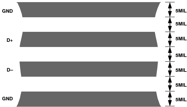
Figure 16. Typical Arrangement of Signal Tracks
