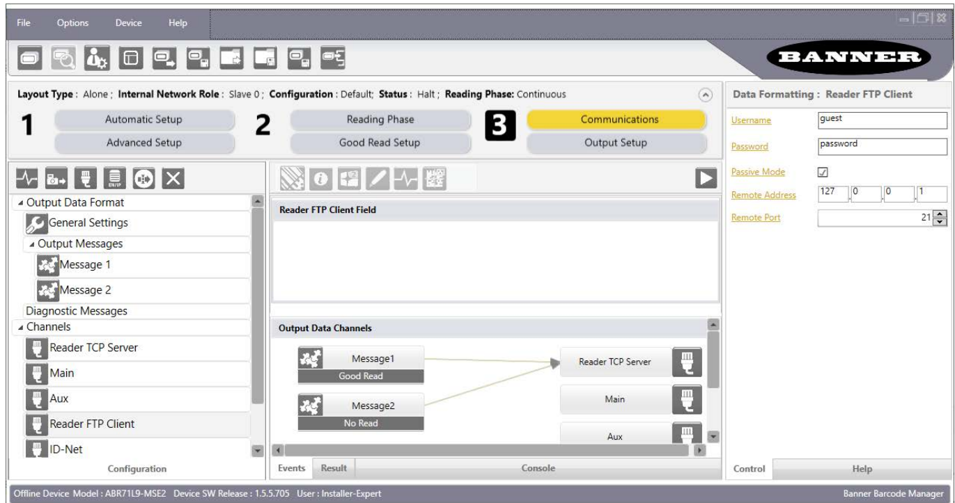
Figure 115. Communications: Reader FTP Client
