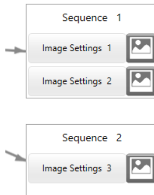
Figure 34. Multiple Image Settings in one Acquisition Sequence
