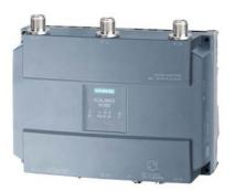
product announced for discontinuation; IWLAN client, SCALANCE W748-1 M12, 1 radio, 3 N-CON antenna port, iFeatures support via KEY-PLUG, IEEE 802.11a/b/g/h/n, 2.4/5GHz, gross 450 Mbps per radio, 1x M12 max. 1 Gbps, PoE, redundant 24 V DC,M12 A-coded IP65, -20..+60 °C, plug slot, WPA2/802.11i/e, signaling contact observe national approvals! cert ID: RAPN-W1-M12-E3, includes: MPCIE-R1-ABGN-U3, scope of delivery: manuals on CD-ROM, German/English; M12 sealing caps, for operation in the USA.
