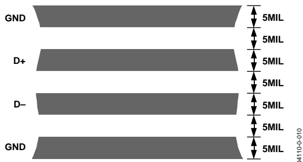
Figure 24. Typical Arrangement of Signal Tracks
