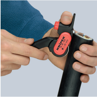
Setting the tool for longitudinal cut
