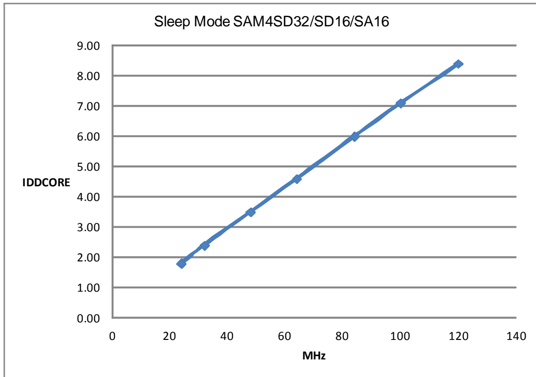
Figure 44-8. SAM4SD32/SD16/SA16 Typical Current Consumption in Sleep Mode (AMP1) vs Master Clock Ranges (refer to Table 44-16)
