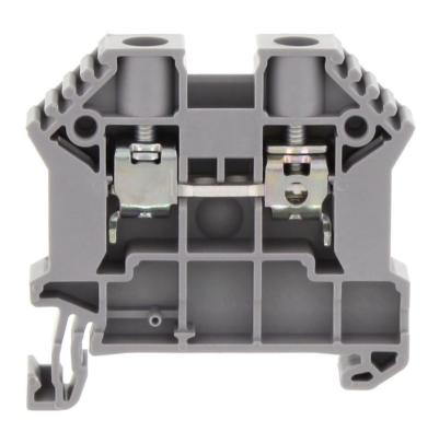
Feed-through terminal, Screw connection, Mounting type: Mounting rail TS 35/7.5, Rated cross-section: 10 mm², Width: 8 mm, Colour: Grey
