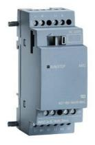
SIPLUS LOGO! AM2 based on 6ED1055-1MA00-0BA2 with conformal coating, -40...+70 °C, start up -25 °C, expansion module, PS/: 12/24 V DC, 2 AI, 0-10 V or 0/4-20 mA for LOGO! 8
