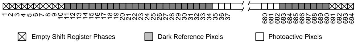
Figure 13. Line Timing Diagram – Single Register Output
