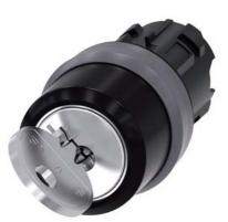
RONIS key-operated switch, 22 mm, round, plastic with metal front ring, lock number SB30, with 2 keys, 2 switch positions O<I, momentary contact type, Actuating angle 45°, 10:30h/12h, key removal O, possible special locks: SB31, 421, 455, with laser labeling, upper case
