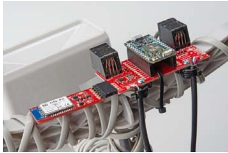
A SparkFun BlueSMiRF Silver connected to the Serial 1 Port using a 6-pin, right-angle female header with the outermost pins removed.
