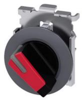
Selector switch, illuminable, 30 mm, round, Metal, matte, red, selector switch, short, front ring for flush installation, 2 switch positions O<I, momentary contact type, Actuating angle 45°, 10:30h/12h, with laser labeling, upper case and lower case, always upper case at the beginning of the word
