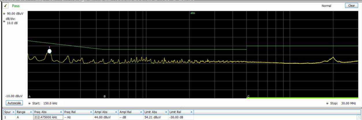
EMI; Conducted CISPR 22; Peak vs. Average Limit; L2/Neutral; 208Vac 24Vdc @ 25Adc
