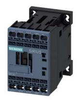
power contactor, AC-3 7 A, 3 kW / 400 V 1 NO, 110 V AC, 50 Hz 120 V, 60 Hz, 3-pole, Size S00, Spring-type terminal Multi-unit packaging = 32 units
