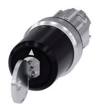
key-operated switch Siemens, 22 mm, round, metal, shiny, lock no. STGH10, with 2 keys, 3 switch positions I>O<II, momentary contact type, actuating angle  $2x45^{\circ}$ , 10:30h/12h/13:30h, key removal O, with laser labeling, upper case and lower case, always upper case at beginning of line
