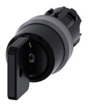
Key-operated switch O.M.R, 22 mm, round, plastic with metal front ring, lock number 73034, black, with 2 keys, 3 switch positions I>O<II, momentary contact type, actuating angle 2x45°, 10:30h/12h/13:30h, key removal O, with laser labeling, upper case and lower case, always upper case at beginning of line
