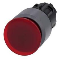
Illuminated mushroom pushbutton, 22 mm, round, plastic with metal front ring, red, 30 mm, latching, pull-to-unlatch mechanism, with laser labeling, inscription or symbol Customer-specific selection with SIRIUS ACT configurator (CIN)
