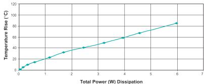
Total Power Dissipation (W) = .001 \* (DCRprimary \* IRMs\_primary² + DCRsecondary \* IRMs\_secondary²) + Core Loss (W)
