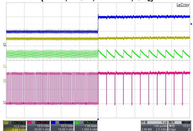
LED short protection(Vin=20V, 3LEDs) (Y-Vin, R-SW, B-LED K, G-I L )
