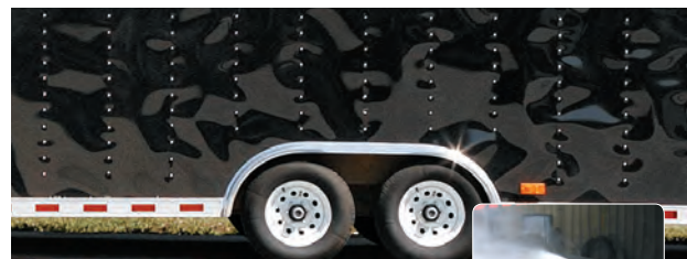
Mechanically fastened at 36,000 miles — leaks at less than 75 psi.
