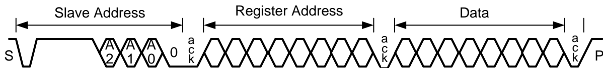
Figure 35. Serial Control Bus: WRITE
