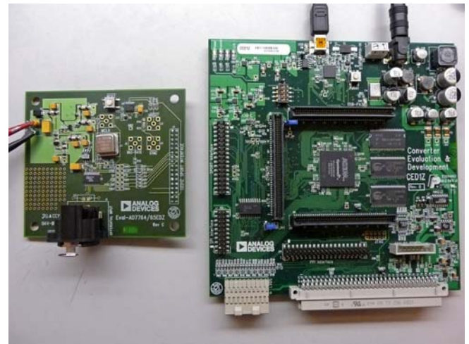
Figure 9. Lining up EVAL-AD7764/65EDZ with the EVAL-CED1Z SPORT connector. Both boards are powered up.
