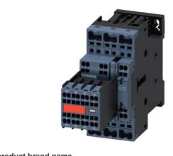
Contactor, AC-3, 18.5 kW / 400 V, 2 NO + 2 NC, 110 V AC, 50 Hz, 120 V, 60 Hz, 3-pole, Size S0, Spring type terminal Captive auxiliary switch
