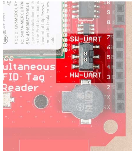
UART Selection Switch Set to SW-UART.
