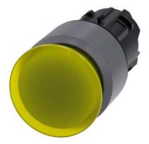
Illuminated mushroom pushbutton, 22 mm, round, plastic with metal front ring, yellow, 30 mm, latching, pull-to-unlatch mechanism, with laser labeling, upper case and lower case, always upper case at beginning of line
