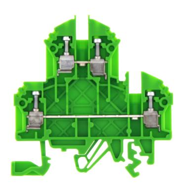
Double-level terminal, Screw connection, Mounting type:Mounting rail TS 35/7.5 and TS 32, Rated cross-section: 2.5 mm², Width: 5 mm, Colour: Green
