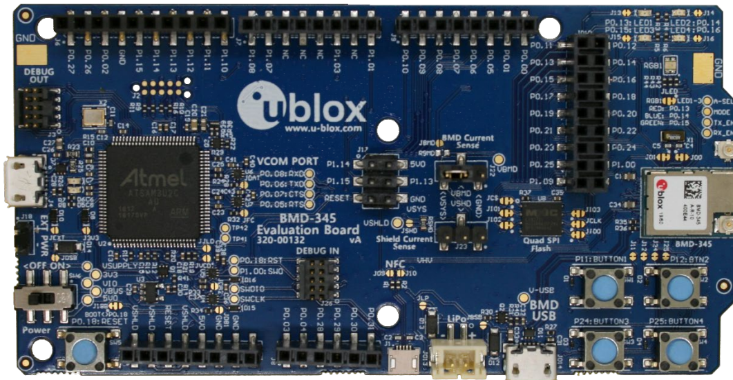
Figure 1: EVK BMD-345 evaluation board (Top view)
